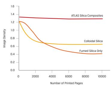
\* Print performance measured with a mono-component printer using model formulations consisting of polyester toner with 325 m<sup>2</sup>/g fumed silica. ATLAS silica composite or colloidal silica were added as spacer particles, as noted. Wt% loading of spacer particles were adjusted to ensure full toner coverage for all formulations.
