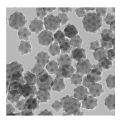
ATLAS 100 silica composite is a breakthrough material for electrophotography applications. It is comprised of hydrophobic silica and polymer in spheroid particles of approximately 100 nm in diameter. The shape and size of ATLAS silica composite particles have been engineered to prevent embedding, migration, and separation from the toner surface.
